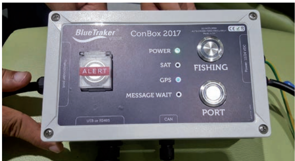
A new BlueTraker unit that is designed to be installed in the bridge. This unit includes port, fishing, and SOS alert functions.
