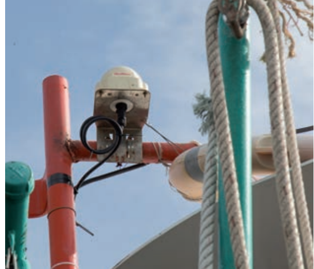
Two examples of MTU showing the new steel cable locking mechanism. © EJF
