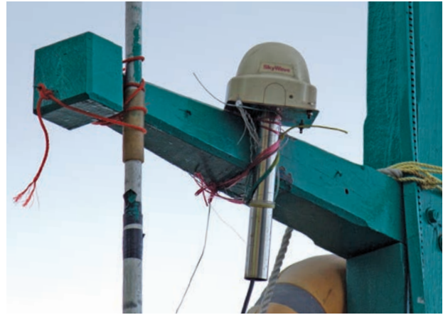
Two examples of MTUs showing a well-fixed MTU with steel locking mechanism (left) and on the right, an MTU which is only loosely secured with string.
