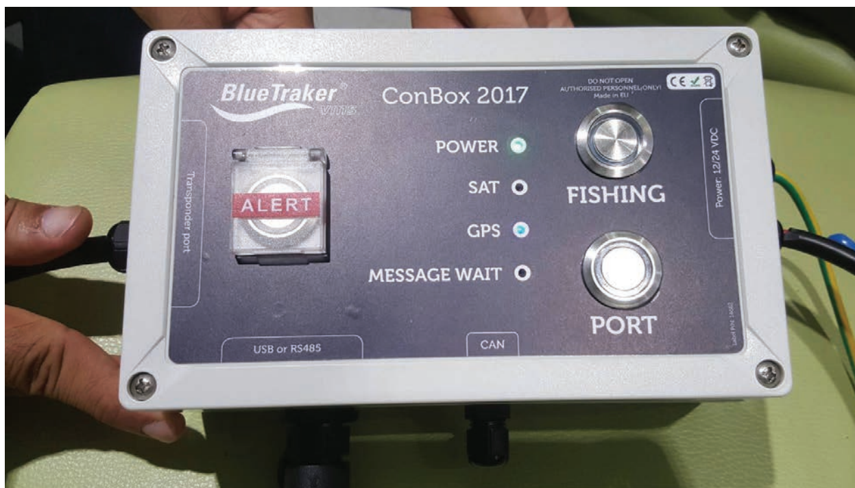
A new BlueTraker unit that is designed to be installed in the bridge. This unit includes port, fishing, and SOS alert functions.
