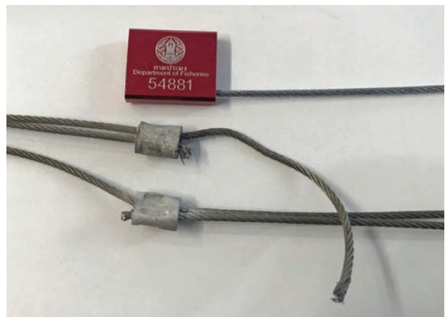
These photos show the steel locking mechanism attached to a VMS MTU (left) and a degraded lock (right).
