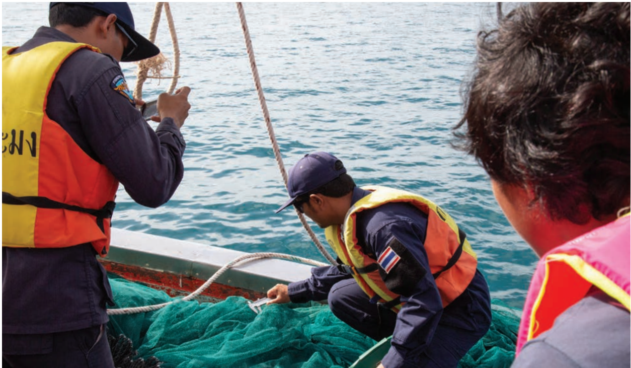
A DoF official measures the mesh size of the net to ensure it is in accordance with the regulations.
