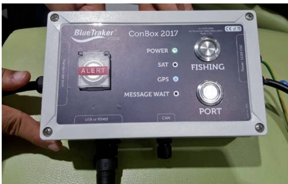
A new BlueTraker unit that is designed to be installed in the bridge. This unit includes port, fishing, and SOS alert functions.
