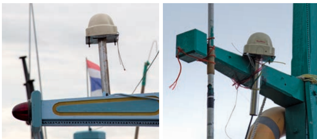
Two examples of MTUs showing a well-fixed MTU with steel locking mechanism (left) and on the right, an MTU which is only loosely secured with string. © EJF
