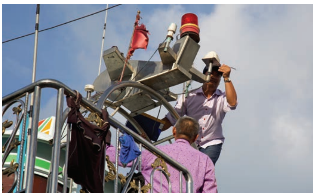
A PIPO official inspects the anti-tampering device fitted to the vessel's VMS unit – an integral part to any PIPO inspection. © EJJ
