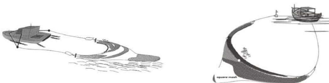
JHIK commonly used for mid-trawling (left) and JTK commonly used for bottom trawling (right)
