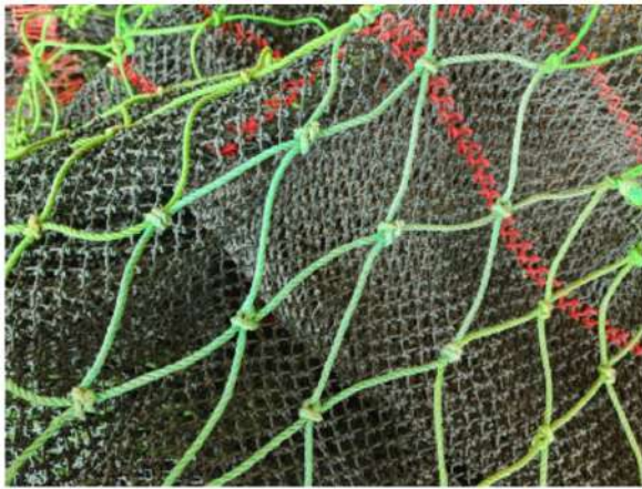
Illegal fishing gear modification (violating MMAF Regulation No. 18 of 2021, 25(3) on JTK and article 26(2) and 27 on JHIK): an addition of one-inch sized double pouch at the top of the net (left); a two inches net without a double pouch (right). Photographed in Batang, Central Java.
