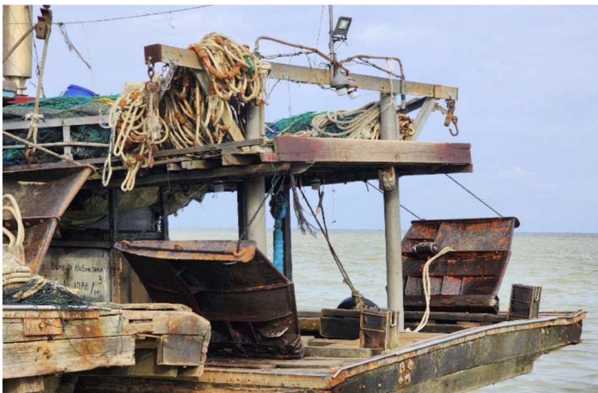
This vessel is fitted with board-shaped iron ballasts at the bow section – an illegal practice.
