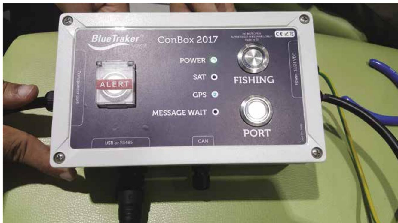
An example of a new Gen 2 unit incorporating new port, fishing, and SOS alert functions.
