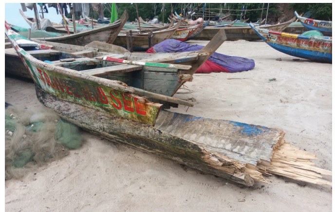
Sections of a canoe destroyed upon collision with an industrial vessel at Senya Beraku © Hen Mpoano
