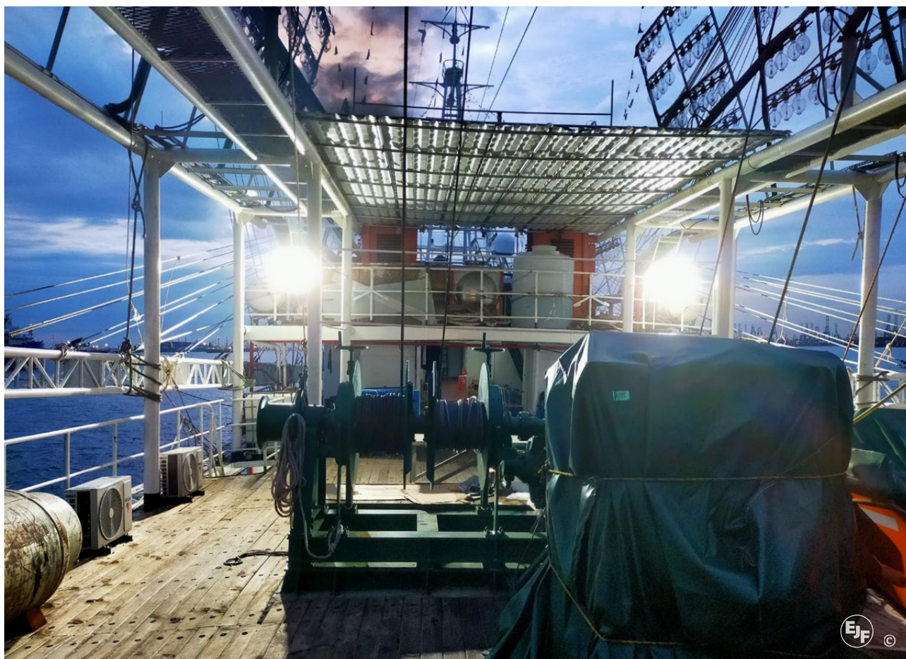
Lighting rigs on a Chinese-flagged light seiner operating in the Northwest Indian Ocean.
