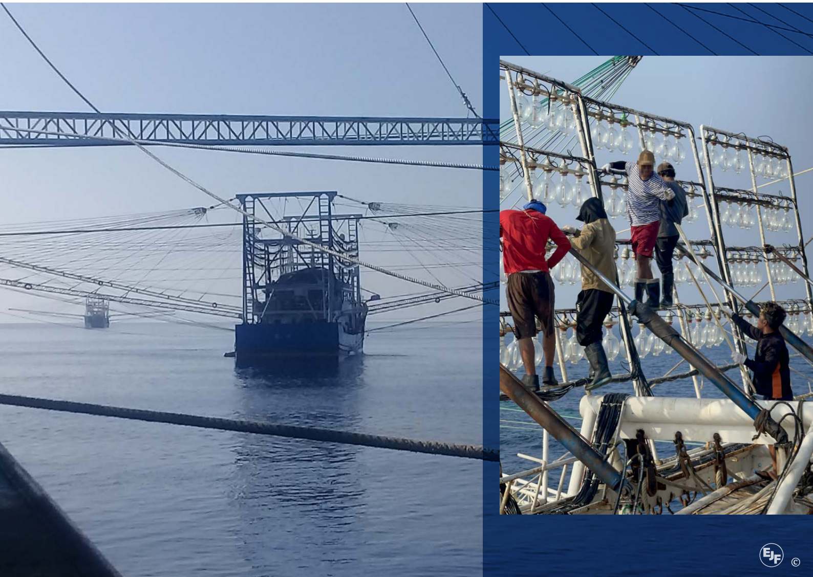
Photos taken onboard Chinese-flagged light seiners in the NWIO. (Left) Two light seiners in the distance. The booms that carry the net along with the vessel superstructure, which holds the high-powered light rigs, are all visible. (Right) Fishers perform maintenance on the lights of a light seiner.
