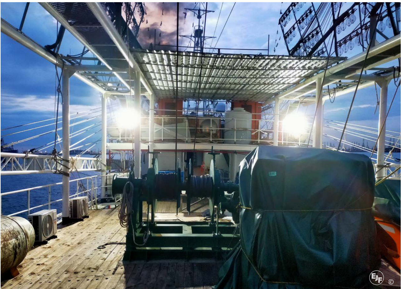
Lighting rigs on a Chinese-flagged light seiner operating in the Northwest Indian Ocean.
