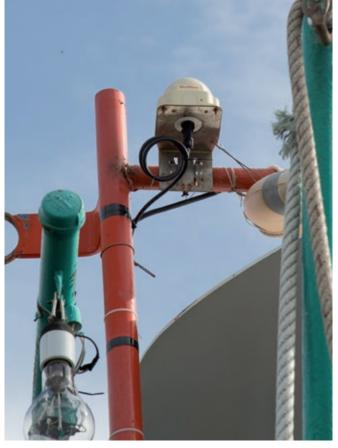
Two examples of MTU showing the new steel cable locking mechanism. © EJF
