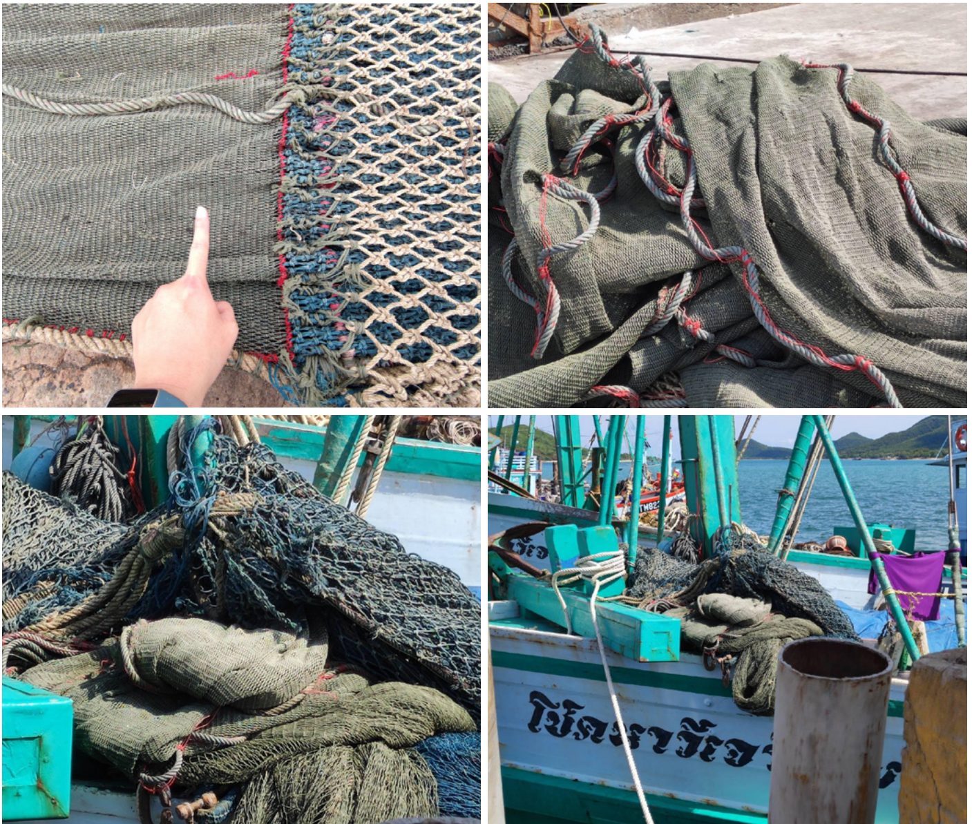
Figure 18: (Clockwise from top left) A legal net used by pair trawlers shows how the body of the net has a significantly finer mesh size than the cod-end of the net. (Top right) Cleaned net ready for installation. (Bottom right & left) Clean nets obscure finer mesh nets underneath.
